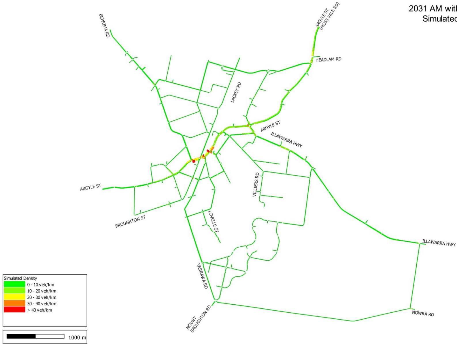
Figure 9-3 2031 with bypass network density (AM)
