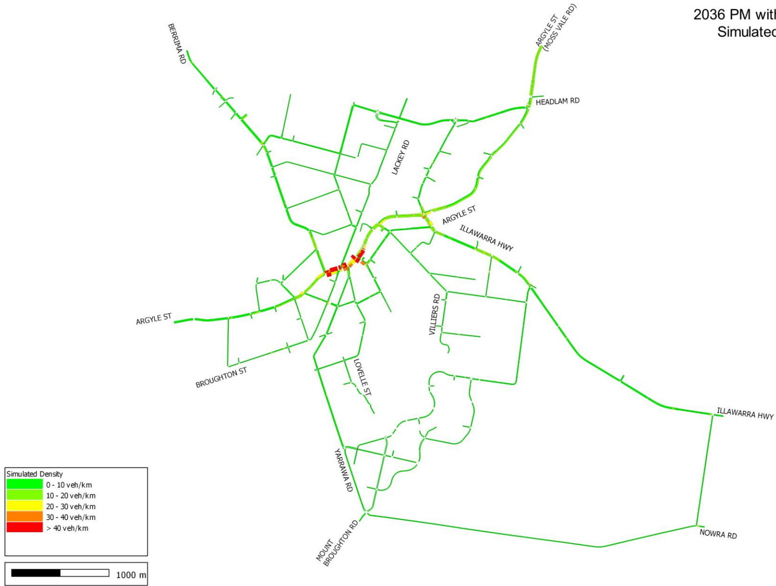
Figure 9-6 2036 with bypass network density (PM)
