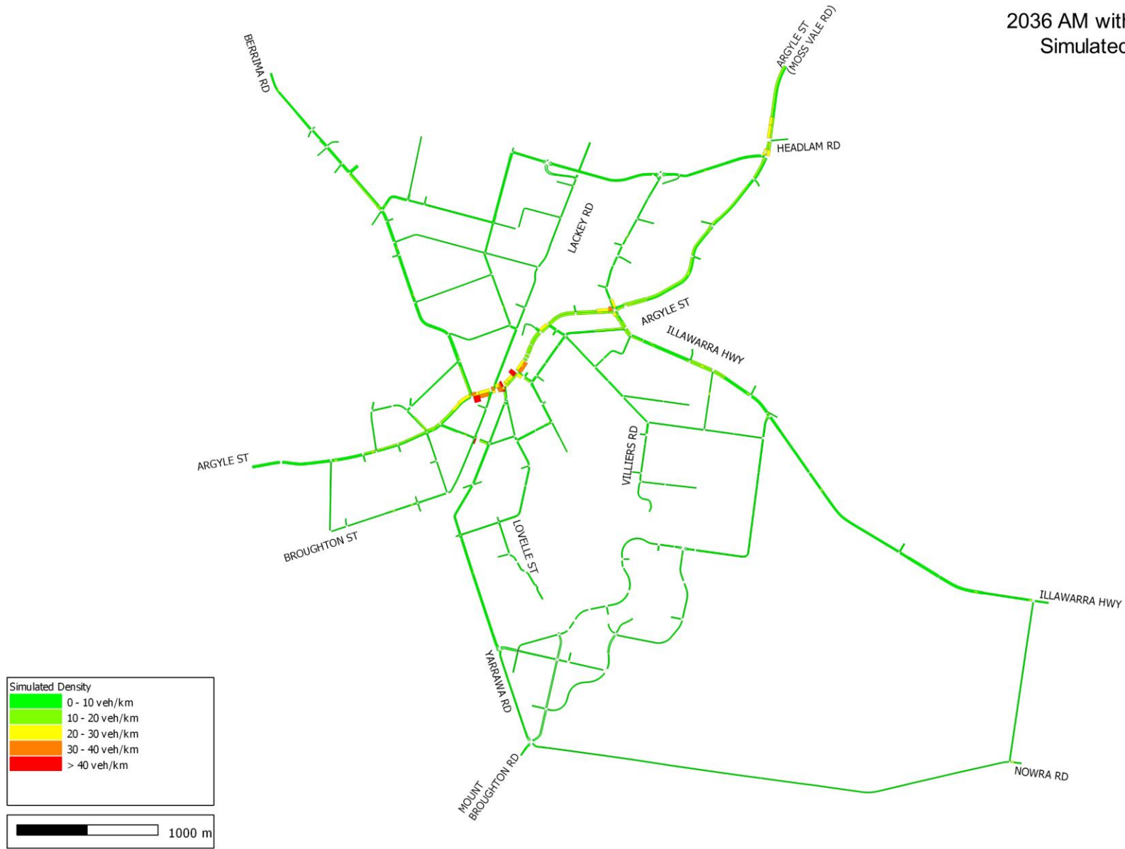
Figure 9-5 2036 with bypass network density (AM)
